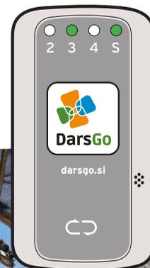
The DarsGo unit will register the vehicle registration number and EURO emission class, and the toll class will be specified by the driver before each trip with respect to the number of vehicle axles.
